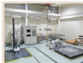
As a means of accommodating increased globalization, we introduced a drop testing machine used to confirm that the packaging is safe even if the product is dropped or impacted during transport.
