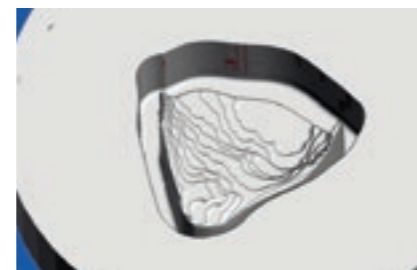
Virtually simulated milling with 3D model.
