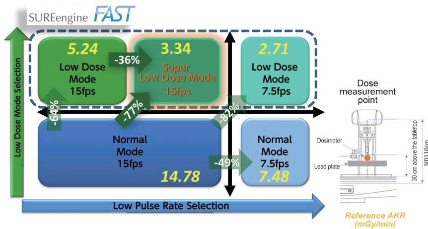
**Fig.8** Comparison of Radiation Dose (AKR) for Each Fluoroscopy Mode
